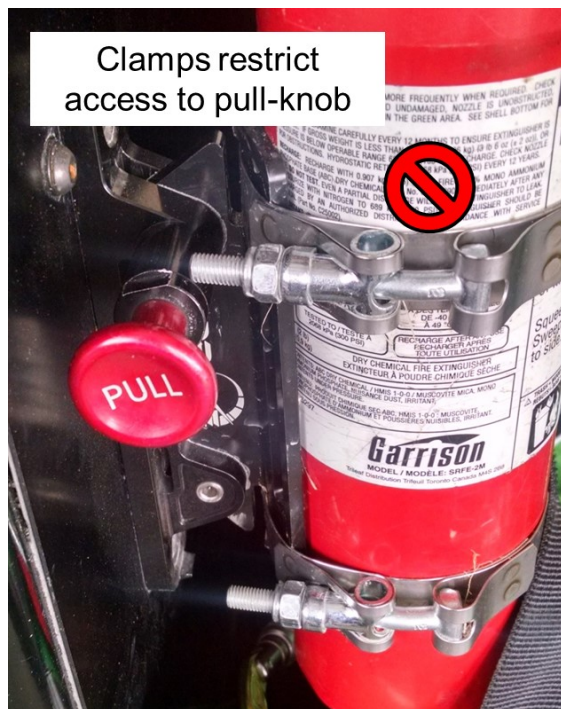
Figure B-47: Incorrect orientation of extinguisher clamps.
