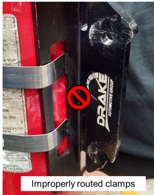
Figure B-52: Incorrect routing of hose clamps.
