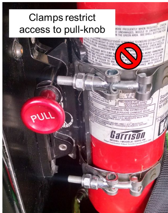
Figure B-51: Incorrect orientation of extinguisher clamps.
