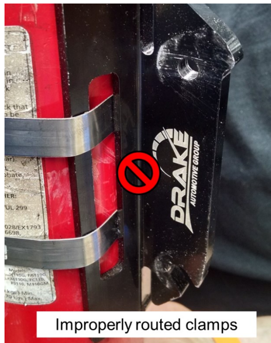
Figure B-47: Incorrect routing of hose clamps.
