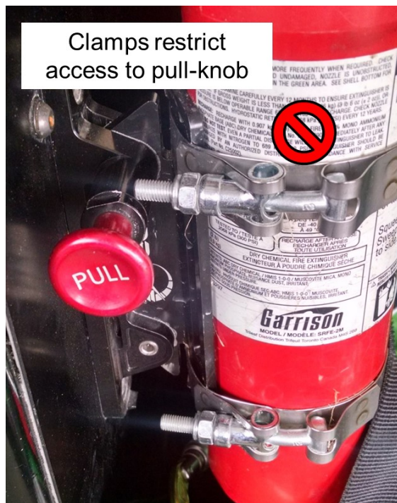
Figure B-46: Incorrect orientation of extinguisher clamps.
